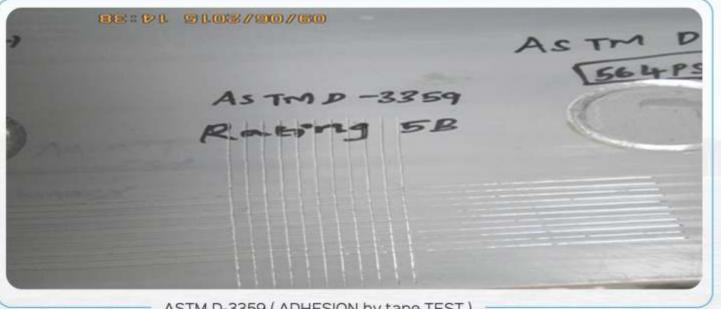
ASTM D-3359 (ADHESION by tape TEST)
